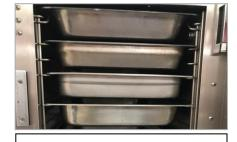
Load steamer starting from the top rack, placing the next pan on the rack directly below, until all pans are loaded.
